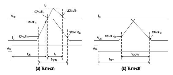
Figure 4. Switching Time Definition
