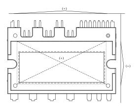
Figure 6. Flatness Measurement Position
