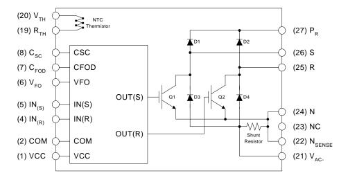
Figure 3. Internal Block Diagram
