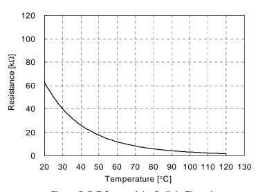
Figure 5. R-T Curve of the Built-in Thermistor
