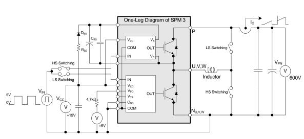
Figure 5. Example Circuit for Switching Test
