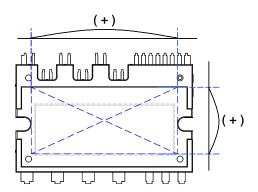
Figure 9. Flatness Measurement Position
