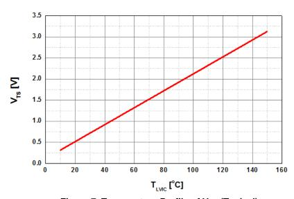
Figure 7. Temperature Profile of V<sub>TS</sub> (Typical)
