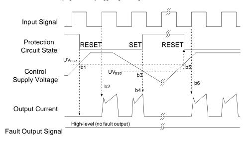
Figure 12. Under-Voltage Protection (High-Side)
