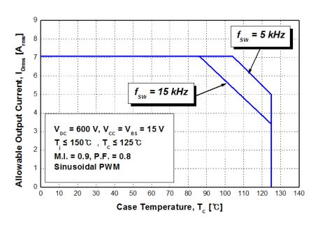
Figure 8. Allowable Maximum Output Current
