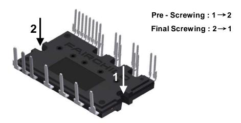
Figure 10. Mounting Screws Torque Order
