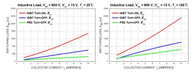
Figure 6. Switching Loss Characteristics
