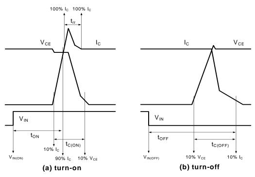
Figure 4. Switching Time Definition
