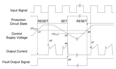
Figure 11. Under-Voltage Protection (Low-Side)
