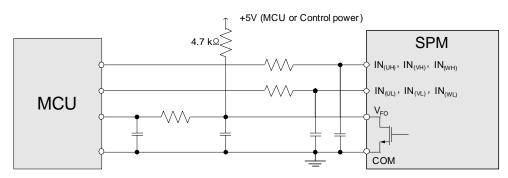
Figure 14. Recommended CPU I/O Interface Circuit
