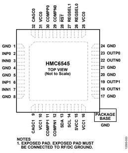
Figure 2. Pin Configuration
