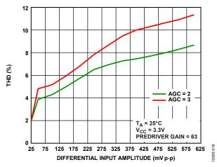
Figure 19. THD vs. Differential Input Amplitude Over AGC Value, Tap 4 Gain Is Set to Maximum Gain, While Others Are Enabled with No Gain
