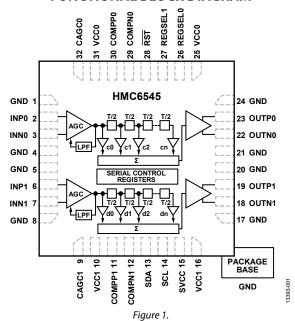
input of the FFE. The 9-tap FFE is programmed via 2-wire interface to generate wide range frequency responses that are precursor or postcursor in nature for compensating signal impairments. After FFE tap coefficients are summed at the summing node, the signal is received by a linear output driver. DC offset correction circuitry is controlled either automatically or manually via Forward Error Correction (FEC).
