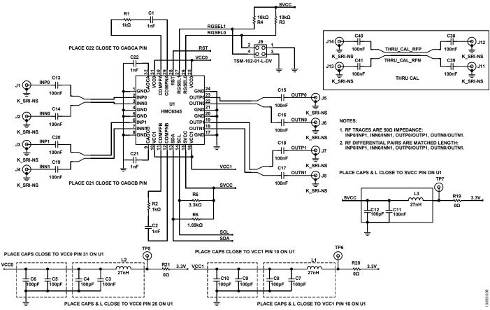
Figure 35. Evaluation Board Schematic
