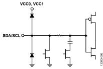
Figure 7. SDA, SCL Interface Schematic
