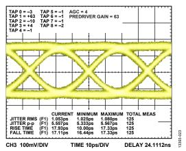
Figure 24. Typical Output Waveform t 28 Gbps, PRBS 2<sup>31</sup> – 1 Input Data
