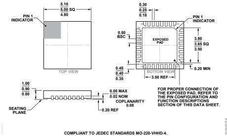
Figure 36.32-Lead Lead Frame Chip Scale Package [LFCSP] 5 mm × 5 mm Body and 0.90 mm Package Height (HCP-32-1) Dimensions shown in millimeters
