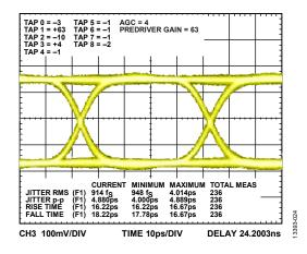
Figure 25. Typical Output Waveform at 10 Gbps PRBS 2<sup>31</sup> – 1 Input Data
