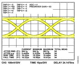
Figure 23. Typical Output Waveform at 22 Gbps, PRBS 2<sup>31</sup> – 1 Input Data, Input Signal = 300 mV p-p Differential
