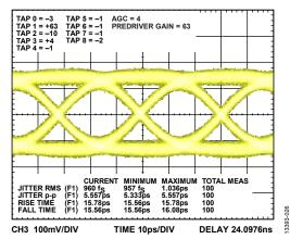
Figure 27. Typical Output Waveform at 32 Gbps, PRBS 2<sup>31</sup> – 1 Input Data
