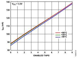
Figure 13. Supply Current vs. Enabled Taps Over Temperature
