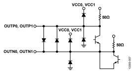
Figure 8. OUTPx, OUTNx Interface Schematic
