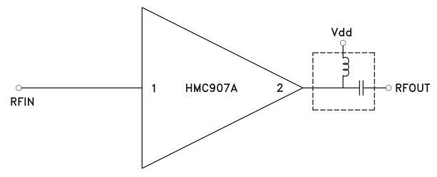
NOTE 1: Drain Bias (Vdd) must be applied through a broadband bias tee with low series resistance and capable of providing 500mA
