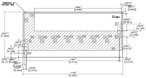
This die utilizes fragile air bridges. Any pick-up tools used must not contact the die in the cross hatched area.
