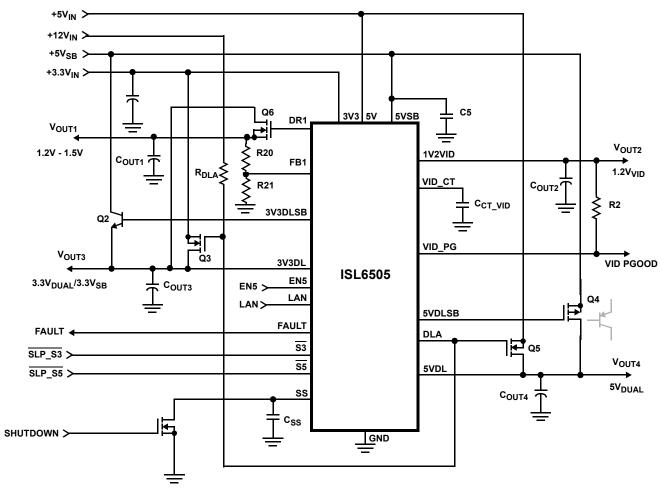
$V_{OUT1} = 1.2V \text{ to } 1.5V: Q6 = FDD6530A, C_{OUT1} = 1000 \mu F$
