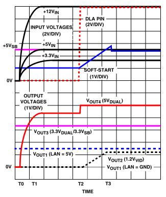
FIGURE 9. SOFT-START INTERVAL IN ACTIVE STATE
