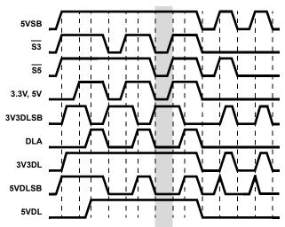
FIGURE 5. 5V<sub>DUAL</sub> AND 3.3V<sub>DUAL</sub>/3.3V<sub>SB</sub> TIMING DIAGRAM; EN5 = 5V/OPEN
