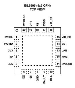
NOTE: The QFN bottom pad is electrically connected to the IC substrate, at GND potential. It can be left unconnected, or connected to GND; do NOT connect to another potential.
