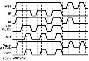
FIGURE 6. V<sub>OUT1</sub> AND 1.2V<sub>VID</sub> TIMING DIAGRAM (NOTE THE DEPENDENCE OF V<sub>OUT1</sub> ON THE LOGIC STATE OF LAN PIN)
