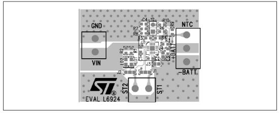
Figure 29. Demonstration board layout, bottom side
