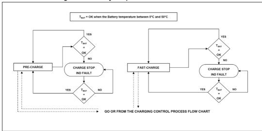
Figure 19. Battery temperature control flow chart
