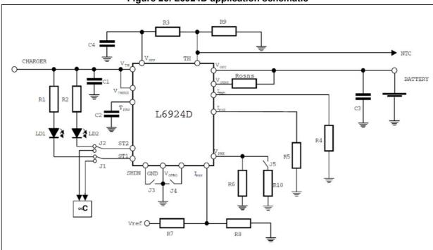
Figure 25. L6924D application schematic
