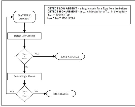
Figure 22. Battery absent detection flow chart
