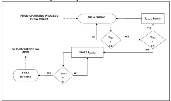
Figure 17. Charge termination flow chart
