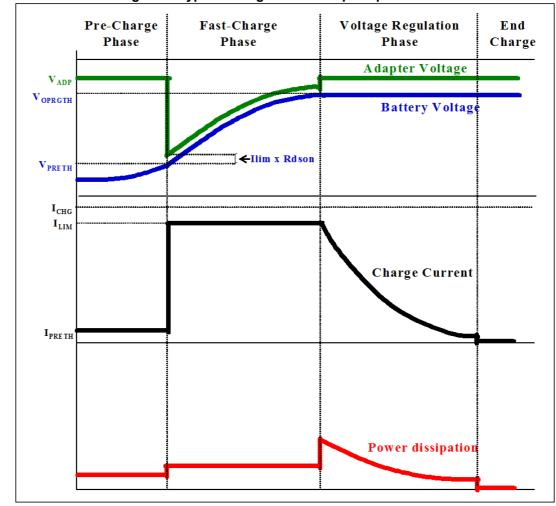
Figure 7. Typical charge curves in quasi pulse mode
