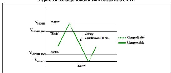
Figure 20. Voltage window with hysteresis on TH
