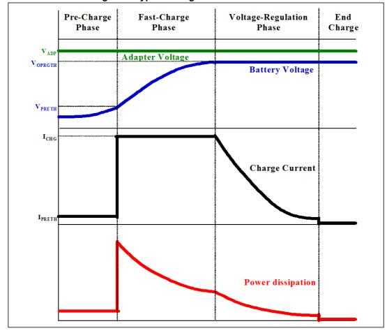
Figure 6. Typical charge curves in linear mode
