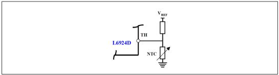
When the TH pin voltage rises and exceeds the  $V_{MINTH}$  = 50% of  $V_{REF}$  (900 mV typ), the L6924D stops the charge, and indicates a fault by the status pins. The device re-starts to charge the battery, only when the voltage at the TH pin goes under  $V_{MINTH\_HYS}$  = 780 mV (typ).
