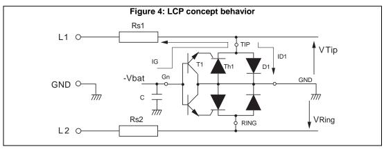
*Figure 4: "LCP concept behavior"* shows the classical protection circuit using the LCP crowbar concept. This topology has been developed to protect the new high voltage SLICs. It allows to program the negative firing threshold while the positive clamping value is fixed at GND.
