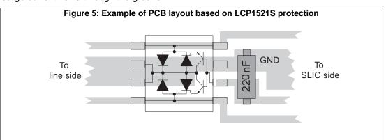
When a positive surge occurs on one wire (L1 for example) the diode D1 conducts and the surge current flows through the ground.
