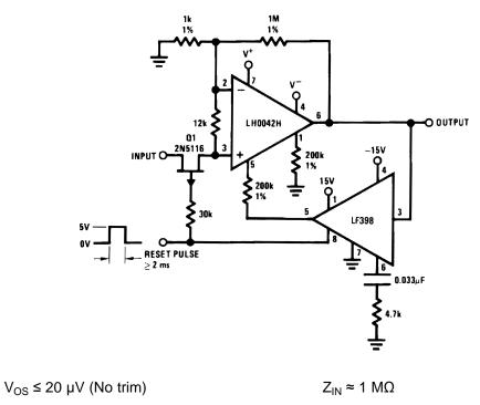
Figure 33. Reset Stabilized Amplifier
