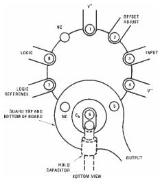
Use 10-pin layout. Guard around C<sub>H</sub> is tied to output.
