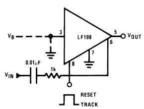
$V_{OUT} = V_B + \Delta V_{IN}$  (HOLD MODE)
