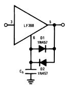
Figure 32. Increased Slew Current
