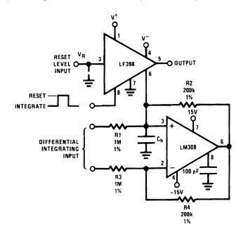
Figure 30. Integrator With Programmable Reset Level
