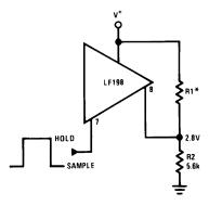
Threshold = 1.4 V Select for 2.8 V at pin 8
