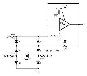
Figure 10. Protecting Op Amp input. The bounding voltage is  $\pm 4V$  with the LM4431 (LM4431's reverse breakdown voltage + 3 diode V<sub>F</sub>).
