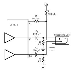
Figure 55. Headphone Sensing Circuit
