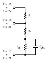
At low, frequencies  $C_{LFE}$  is a virtual open circuit and at high frequencies, its nearly zero ohm impedance shorts  $R_{LFE}$ . The result is increased bridge-amplifier gain at low frequencies. The combination of  $R_{LFE}$  and  $C_{LFE}$  form with a -3dB corner frequency at
