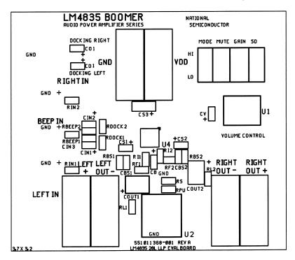
Figure 57. Recommended LQ PC Board Layout: Component-Side Silkscreen
