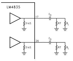
Figure 54. Resistor for Varying Output Loads
