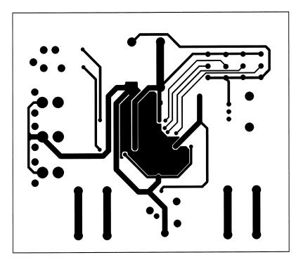
Figure 61. Recommended LQ PC Board Layout: Bottom-Side Layout
