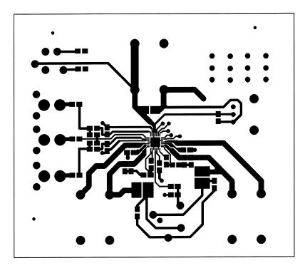
Figure 58. Recommended LQ PC Board Layout: Component-Side Layout
