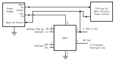
By powering the LM77 from auxilary output of the power supply, a non-functioning overheated computer can be powered down to preserve as much of the system as possible.
