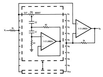
Figure 42. 10 Band Graphic Equalizer
