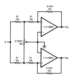
Figure 37. 2 Channel Panning Circuit (Pan Pot)
