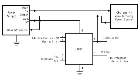
Figure 19. ACPI Compatible Terminal Alarm Shutdown
