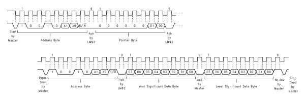
Figure 11. Typical Pointer Set Followed by Immediate Read for 2-Byte Register such as Temp or **Comparison Registers**
