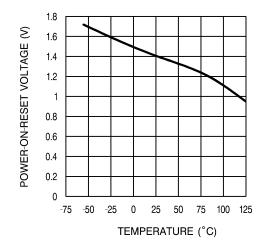
Figure 6. Average Power on Reset Voltage vs Temperature
