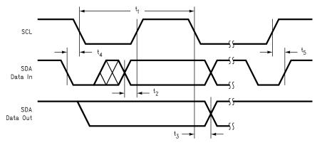
Figure 4. Serial Bus Communication
