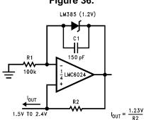
(Upper limit of output range dictated by input common-mode range; lower limit dictated by minimum current requirement of LM385.)
