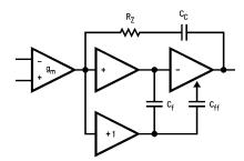
Figure 25. LMC6024 Circuit Topology (Each Amplifier)
