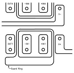
Figure 28. Example of Guard Ring in P.C. Board Layout (Using the LMC6024)
