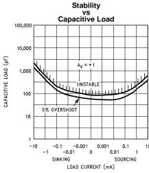
Avoid resistive loads of less than  $500\Omega$ , as they may cause instability. Figure 23.
