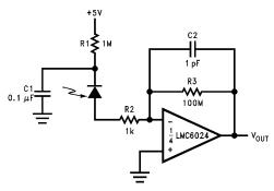
A 5V bias on the photodiode can cut its capacitance by a factor of 2 or 3, leading to improved response and lower noise. However, this bias on the photodiode will cause photodiode leakage (also known as its dark current).
