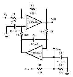
$$\label{eq:Gain} \begin{split} \text{Gain} &= -46.8 \\ \text{Output offset voltage reduced to the level of the input offset voltage of the bottom amplifier (typically 1 mV), referred to $V_{BIAS}$. \end{split}$$
