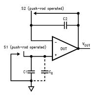
Figure 34. Simple Input Bias Current Test Circuit
