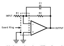
Figure 29. Inverting Amplifier Guard Ring Connections
