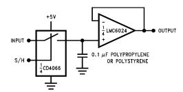
Figure 38. Low-Leakage Sample-and-Hold
