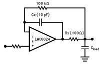
Figure 26. Rx, Cx Improve Capacitive Load Tolerance
