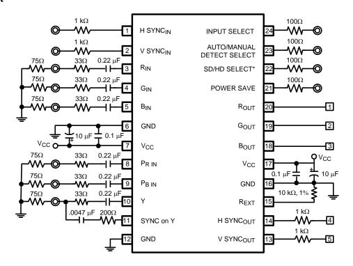
Figure 9. Test Circuit
