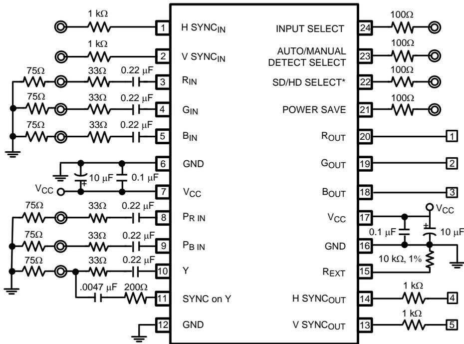
Figure 9. Test Circuit
