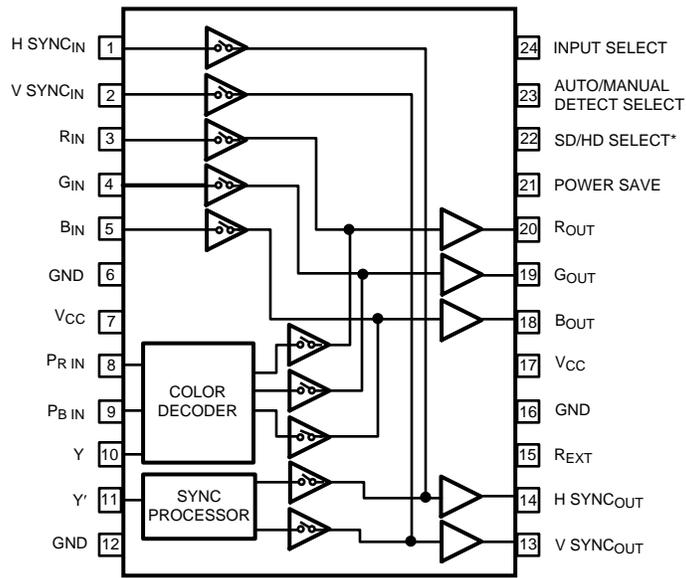
Figure 1. 24-Pin TSSOP - Top View
