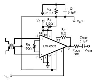
Figure 66. Transformer Coupled Single Supply VGA
