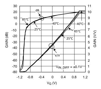
Figure 1. Gain vs. V<sub>G</sub> for Various Temperature
