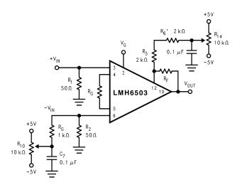
Figure 61. Nulling the Output Offset Voltage
