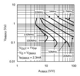
Figure 60. Bandwidth vs. V<sub>INMAX</sub> and A<sub>VMAX</sub>
