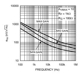
Figure 63. Output Referred Voltage Noise vs. Frequency
