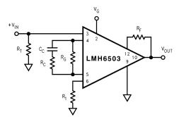
Figure 70. Frequency Shaping
