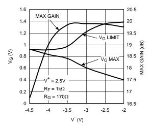
Figure 67.  $V_{G\_MAX}$ ,  $V_{G\_LIMIT}$ , & Max-gain vs.  $V^-$  (V<sup>+</sup> = 2.5V)
