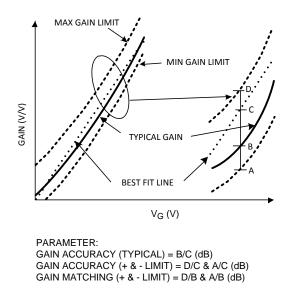
Figure 62. Gain Accuracy and Gain Matching Parameters Defined
