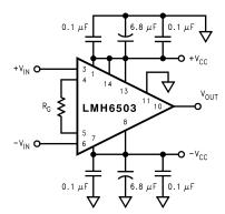
Figure 64. Required Power Supply Decoupling
