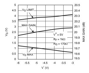
Figure 68.  $V_{G\_MAX}$ ,  $V_{G\_LIMIT}$ , & Max-gain vs.  $V^{-}$ ( $V^{+} = 5V$ )
