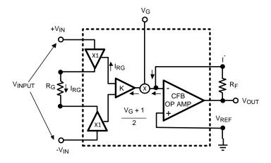
Figure 59. LMH6503 Functional Block Diagram
