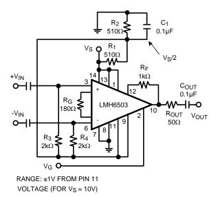
Figure 65. AC Coupled Single Supply VGA
