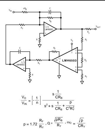
Figure 71. Tunable Bandpass Filter
