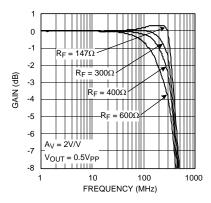
Figure 31. Frequency Response vs. R<sub>F</sub>
