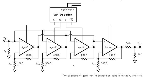
Figure 36. Wideband Digitally Controlled Programmable Gain Amplifier
