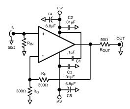
Figure 35. Typical Application with Suggested Supply Bypassing
