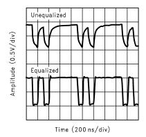
Figure 39. Digital Signal without and with Equalization
