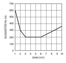
Figure 32. R<sub>F</sub> vs. Non-Inverting Gain
