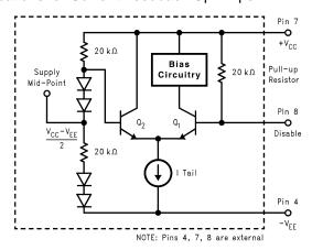
Figure 34. Enable/Disable Operation
