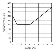
Figure 33. R<sub>F</sub> vs. Inverting Gain
