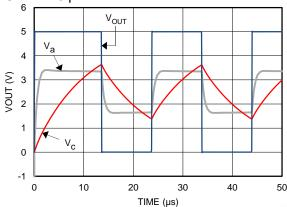
Figure 25. Square-Wave Oscillator Output Waveform
