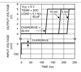
Figure 15. Response Time vs Input Overdrives Positive Transition
