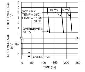
Figure 17. Response Time vs Input Overdrives Negative Transition
