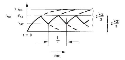
Figure 24. Square-Wave Oscillator Timing Thresholds
