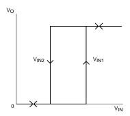
Figure 22. Noninverting Comparator Configuration
