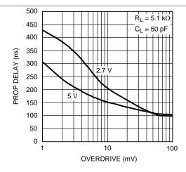
Figure 14. Prop Delay vs Overdrive
