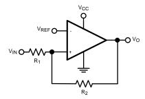
Figure 21. Basic Comparator With Hysteresis
