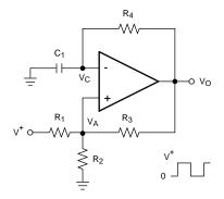
Figure 23. Square-Wave Oscillator
