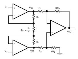
Figure 5. Instrumentation Amplifier
