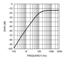
Figure 16. Highpass Filter Frequency Response
