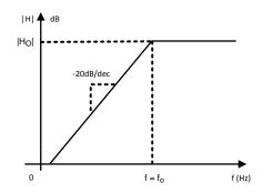
Figure 10. Highpass Filter Transfer Function
