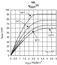
Continuous operation of the device with an output short circuit current larger than 35mA may cause permanent damage to the device.
