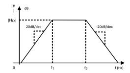
Figure 12. Bandpass filter Transfer Function
