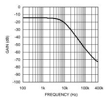
Figure 14. Lowpass Filter Frequency Response
