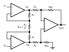
$V_0 = -K (2a + 1) (V_1 - V_2)$  (1)
