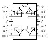
Figure 4. 14-Pin TSSOP (Top View)
