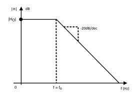
Figure 8. Lowpass Filter Transfer Function
