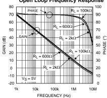
Open Loop Gain & Phase with Cap. Loading
