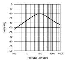
Figure 15. Bandpass Filter Frequency Response
