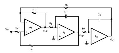
Figure 13. State Variable Active Filter
