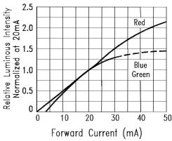
Fig.4 Relative Luminous Intensity vs. Forward Current
