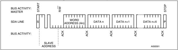
Figure 9. WRITE mode sequence
