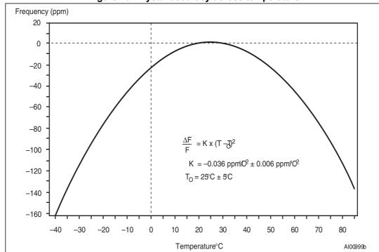
Figure 10. Crystal accuracy across temperature
