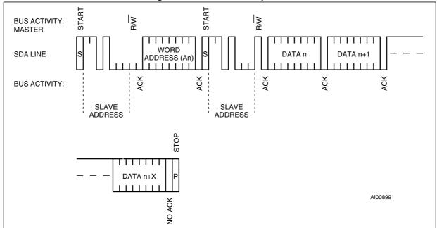
Figure 8. Alternate READ mode sequence
