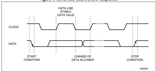
Figure 4. Serial bus data transfer sequence
