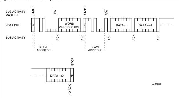
Figure 10. Alternate read mode sequence
