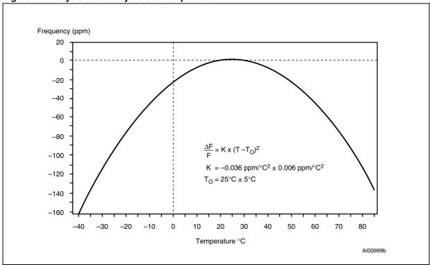
Figure 13. Clock calibration
