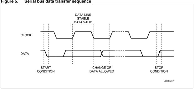
Figure 5. Serial bus data transfer sequence
