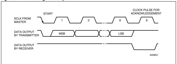
Figure 7. Bus timing requirements sequence
