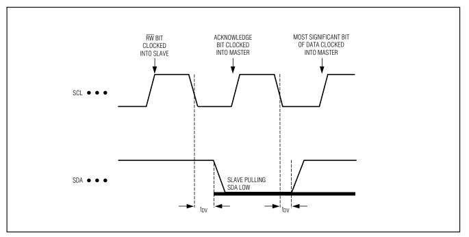
Figure 2. SMBus Serial Interface Timing—Acknowledge
