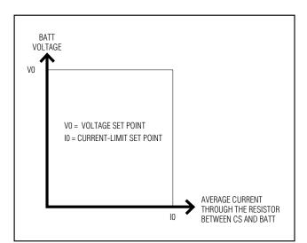
Figure 5. Output V-I Characteristic
