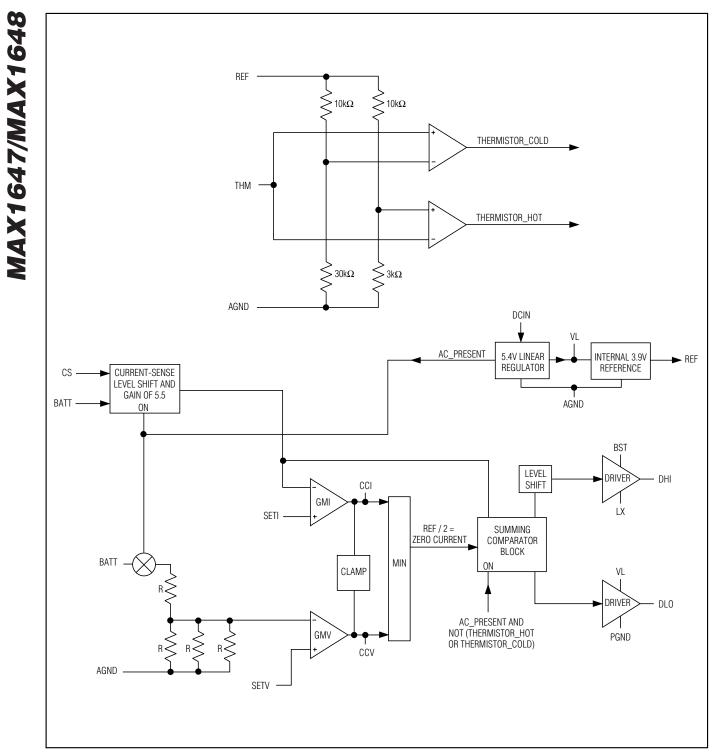
internal current sources' state, and the six most significant bits control the switching regulator's current. The internal current source supplies 1mA resolution to the battery to comply with the smart-battery specification. When the current is set to a number greater than 32, the internal current source remains at 31mA. This guarantees that battery-current setting is monotonic regardless of current-sense resistor choice and current-sense amplifier offset.
