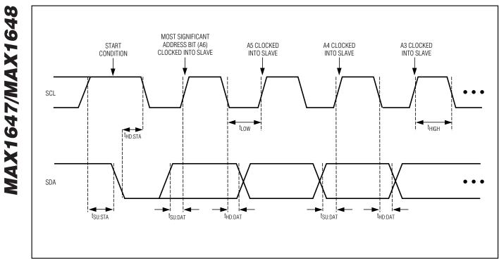
Figure 1. SMBus Serial Interface Timing—Address
