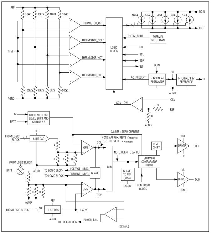
Figure 6a. MAX1647 Block Diagram
