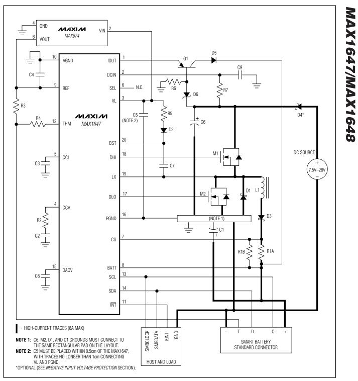
Figure 3. MAX1647 Typical Application Circuit
