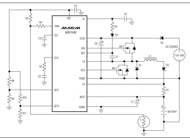
Figure 4. MAX1648 Typical Operating Circuit
