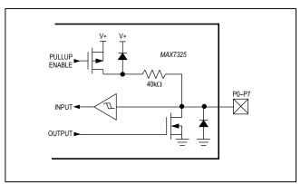
Figure 11. MAX7325 Open-Drain I/O Port Structure
