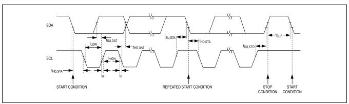
Figure 1. 2-Wire Serial Interface Timing Details
