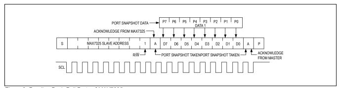
Figure 8. Reading Push-Pull Ports of MAX7325
