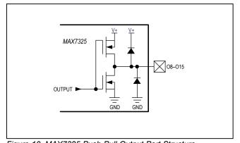
Figure 10. MAX7325 Push-Pull Output Port Structure
