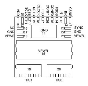
Figure 3. 10XS4200 Pin Assignments
