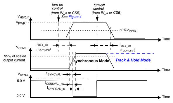
Figure 9. Synchronous & Track-and-Hold Current Sensing Modes: Associated Delay & Settling Times
