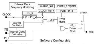
Figure 12. Internal and External Clock Operation
