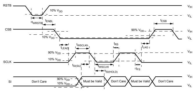
Figure 7. Timing Requirements During SPI Communication
