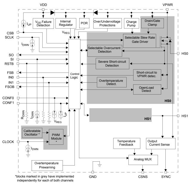
Figure 2. Internal Block Diagram
