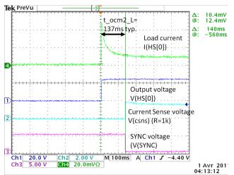
Figure 13. Current Sense Blanking During Overcurrent Window Activity
