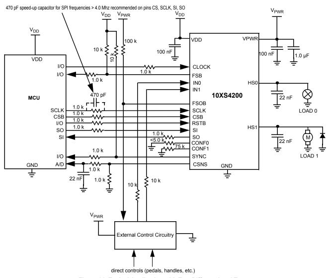
Figure 21. Typical Application with Two Different Load Types
