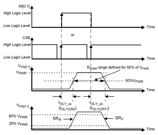
Figure 4. Output Voltage Slew Rate and Delay
