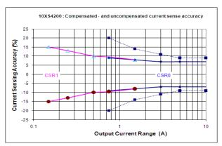
Figure 18. Current Sense Accuracy Versus Output
