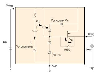
Figure 15. Supply and Output Voltage Protections
