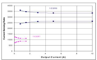
Figure 17. Current Sensing Ratio Versus Output Current
