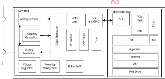
Figure 2. System Level Block Diagram
