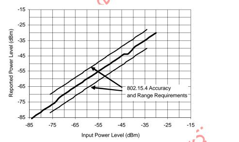
Figure 5. Reported Power Level Versus Input Power for Energy Detect or Link Quality Indicator
