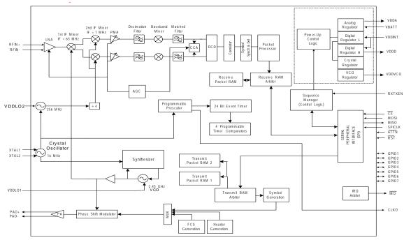
Figure 1. MC13192 Simplified Block Diagram
