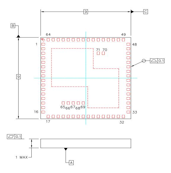
Figure 37. Top View Mechanical (1 of 2)
