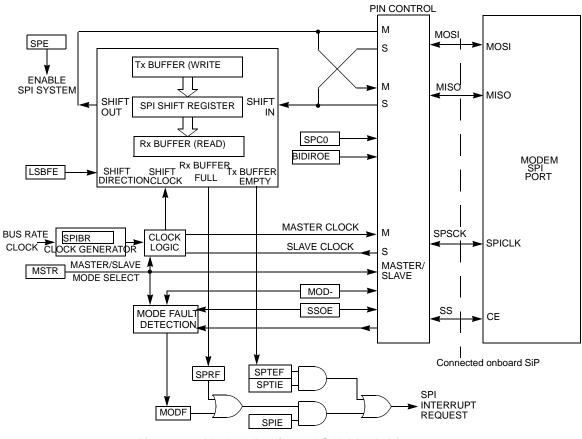
Figure 19. Modem Dedicated SPI Block Diagram
