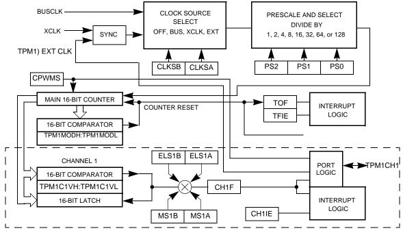
Figure 21. TPM Block Diagram
