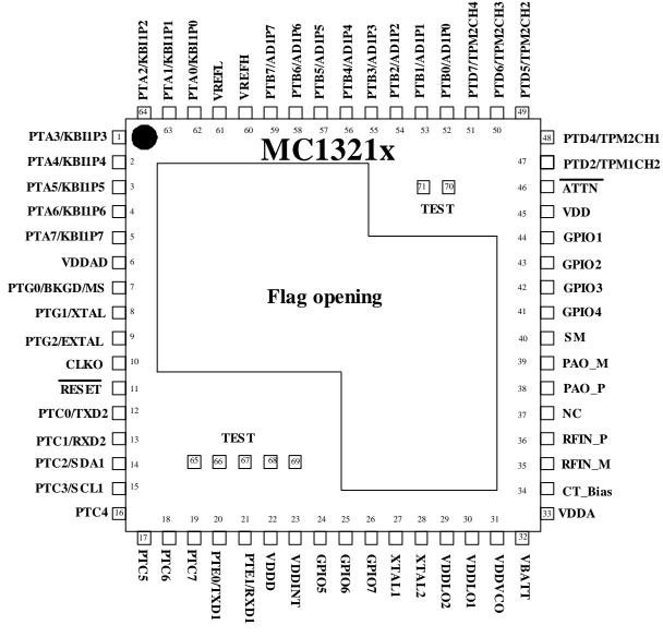
Figure 3. Preliminary MC1321x Pinout
