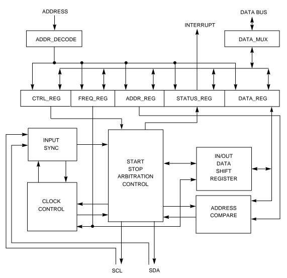
Figure 24. IIC Functional Block Diagram
