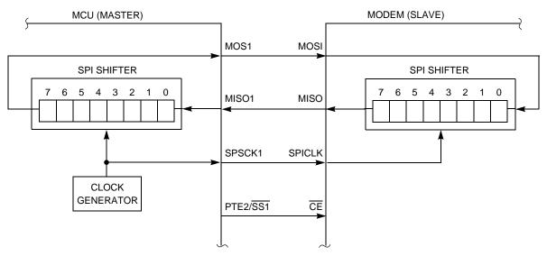
Figure 5. SPI System Block Diagram
