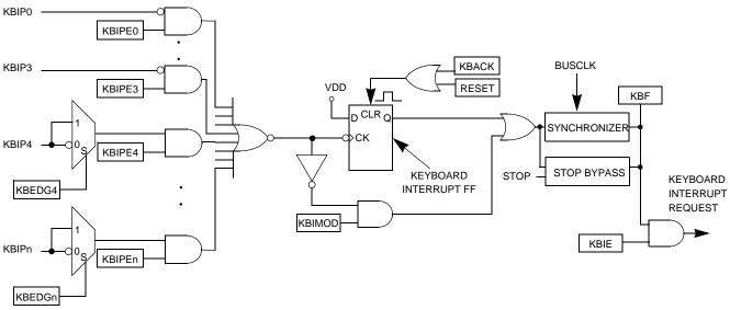
Figure 20. KBI Block Diagram
