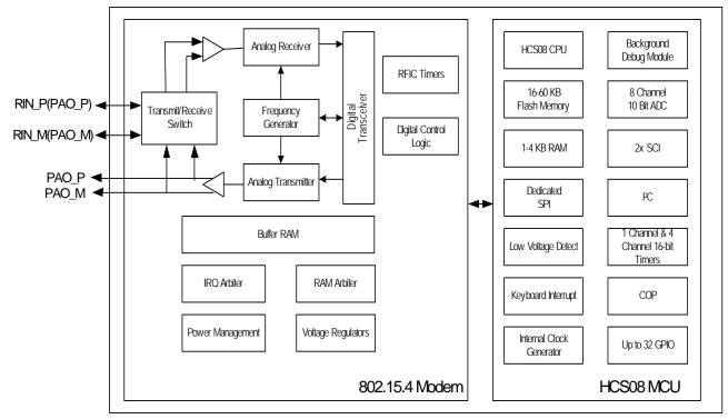
Figure 1. MC1321x System Level Block Diagram
