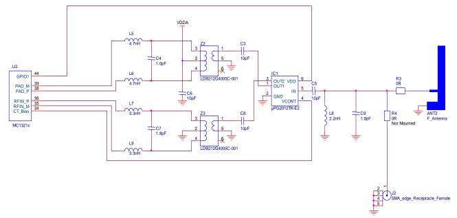
Figure 36. RF Dual Port Application with an F-Antenna
