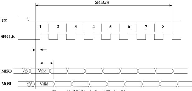
Figure 10. SPI Single Burst Timing Diagram
