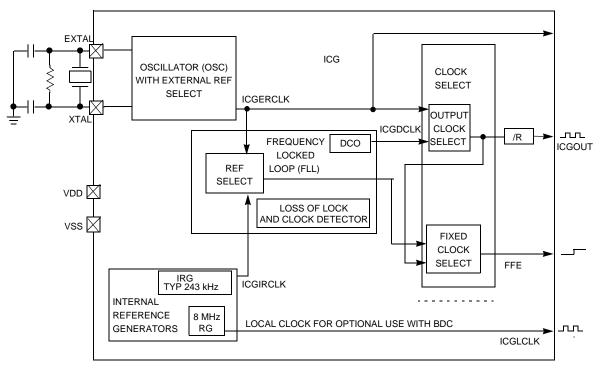
Figure 17. ICG Block Diagram
