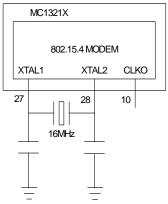
Figure 12. Modem Crystal Oscillator
