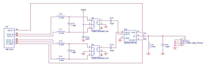
Figure 26. RF Parametric Evaluation Circuit
