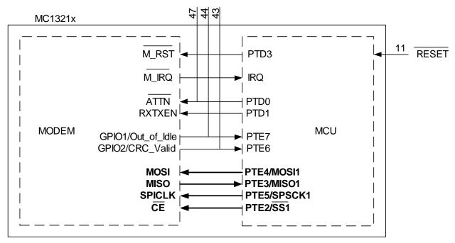
Figure 4. MC1321x Internal Interconnects Highlighting SPI Bus
