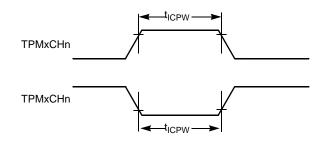
Figure 32. Timer Input Capture Pulse
