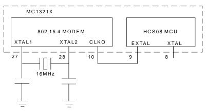
Figure 2. MC1321x Single Crystal System Clock Structure
