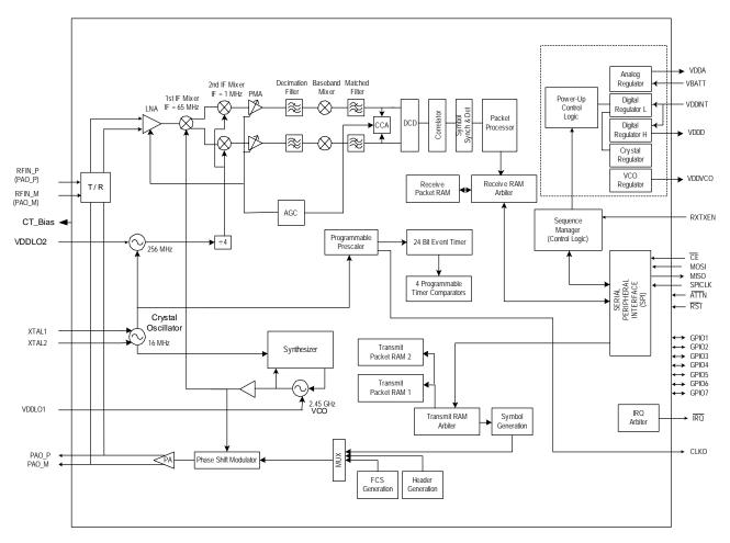
Figure 6. 802.15.4 Modem Block Diagram
