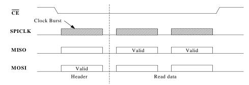
An example SPI read transaction with a 2-byte payload is shown in Figure 11.
