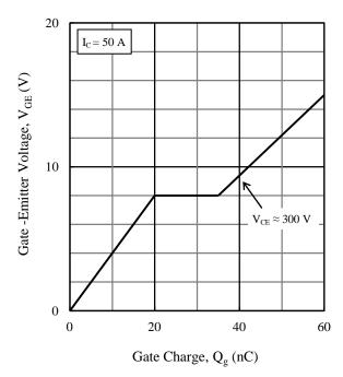
Figure 12. Typical Gate Charge
