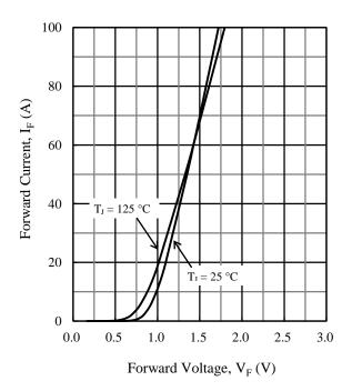
Figure 19. Diode Forward Characteristics
