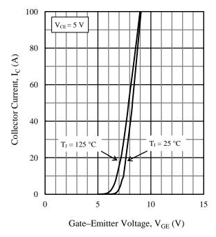
Figure 8. Transfer Characteristics
