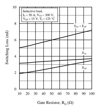
Figure 18. Switching Loss vs. Gate Resistor
