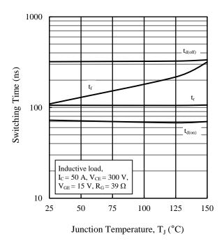
Figure 13. Switching Time vs. Junction Temperature
