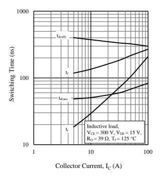
Figure 14. Switching Time vs. Collector Current
