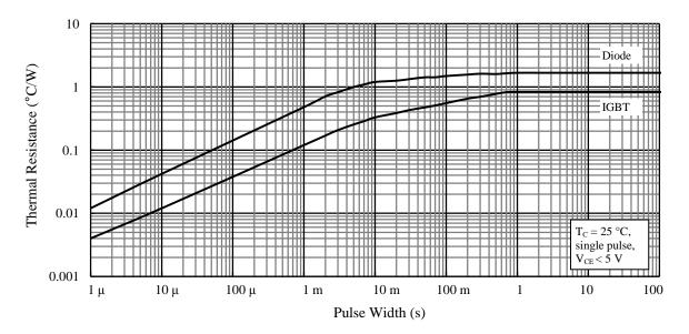
Figure 21. Transient Thermal Resistance
