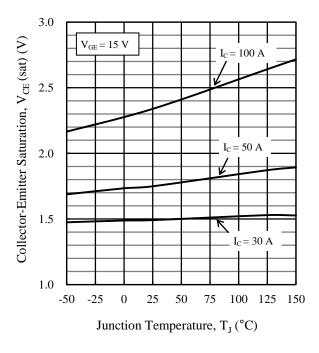
Figure 9. Saturation Voltage vs. Junction Temperature
