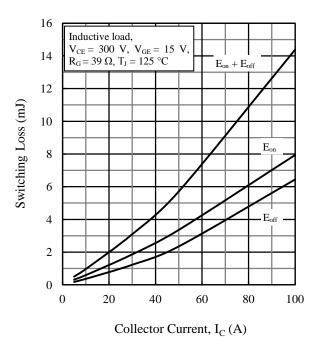
Figure 17. Switching Loss vs. Collector Current
