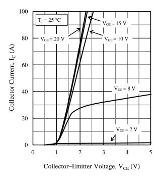
Figure 6. Output Characteristics ( $T_J = 25$  °C)
