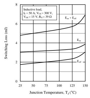
Figure 16. Switching Loss vs. Junction Temperature
