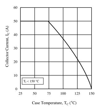
Figure 5. Collector Current vs. Case Temperature
