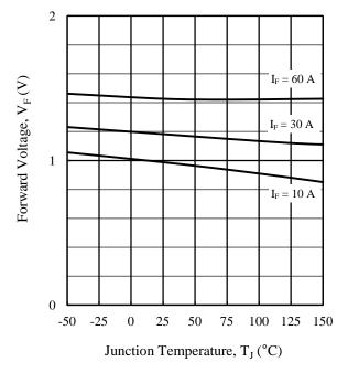
Figure 20. Diode Forward Voltage vs. Junction Temperature
