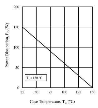
Figure 4. Power Dissipation vs. Case Temperature
