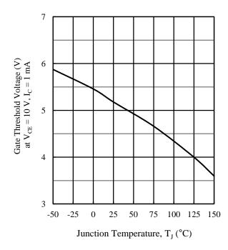
Figure 10. Gate Threshold Voltage vs. Junction Temperature
