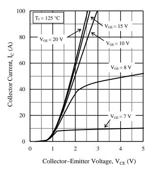
Figure 7. Output Characteristics ( $T_J = 125$  °C)
