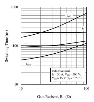
Figure 15. Switching Time vs. Gate Resistor
