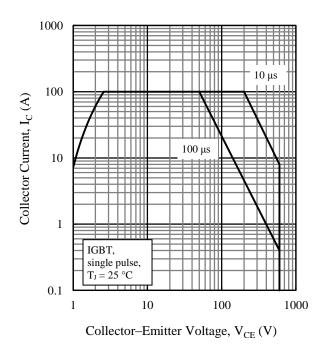
Figure 3. IGBT Safe Operating Area
