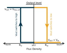
Typically, the device behaves as a latch with symmetric operating and release switching points ( $B_{OP} = |B_{RP}|$ ). This means magnetic fields with equivalent strength and opposite direction drive the output high and low.
