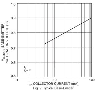
Saturation Voltage vs. Collector Current (PNP-3906)
