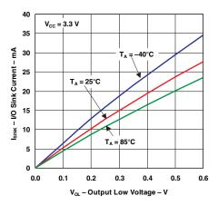
Figure 5. I/O Sink Current vs Output Low Voltage
