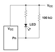
Figure 29. High-Value Resistor In Parallel With The Led
