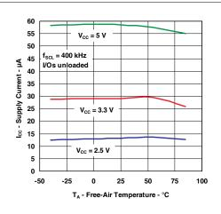
Figure 1. Supply Current vs Temperature
