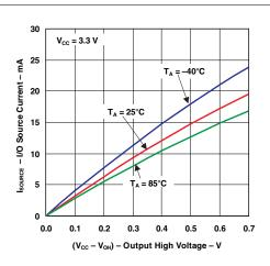
Figure 8. I/O Source Current vs Output High Voltage (P7-P1)
