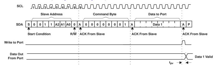
Figure 24. Write To Output Port Register
