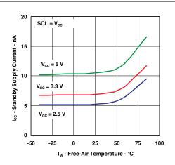
Figure 2. Standby Supply Current vs Temperature
