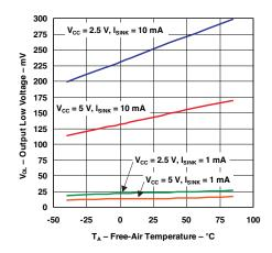
Figure 12. Output Low Voltage vs Temperature
