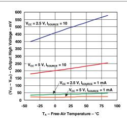
Figure 11. Output High Voltage vs Temperature (P7-P1)
