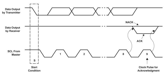
Figure 21. Acknowledgment On The I<sup>2</sup>C Bus
