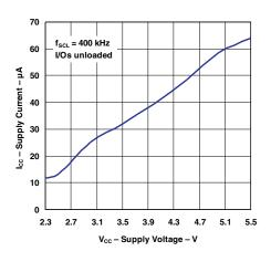
Figure 3. Supply Current vs Supply Voltage
