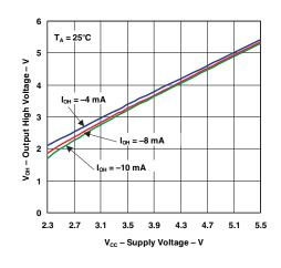
Figure 10. Output High Voltage vs Supply Voltage (P7-P1)
