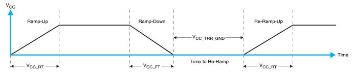
Figure 20. V<sub>CC</sub> is Lowered Below 0.2 V or 0 V and Then Ramped Up to V<sub>CC</sub>
