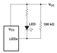
Figure 16. High-Value Resistor in Parallel With LED
