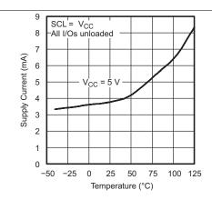
Figure 1. Supply Current vs Temperature
