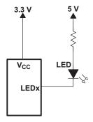
Figure 17. Device Supplied by a Lower Voltage
