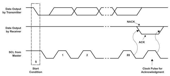
Figure 12. Acknowledgment on I<sup>2</sup>C Bus
