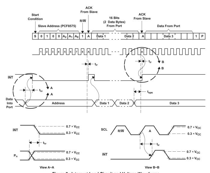
Figure 8. Interrupt Load Circuit and Voltage Waveforms
