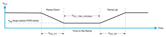
Figure 21. V<sub>CC</sub> is Lowered Below the POR Threshold, Then Ramped Back Up to V<sub>CC</sub>
