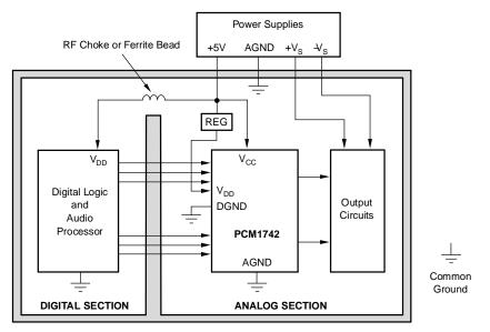
Figure 31. Single-Supply PCB Layout
