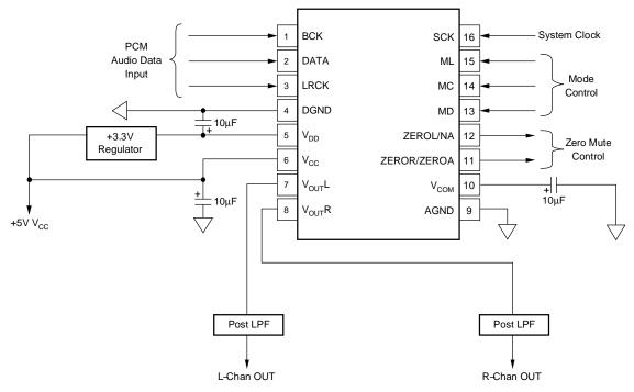
Figure 28. Basic Connection Diagram
