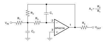
Figure 29. Dual-Supply Filter Circuit
