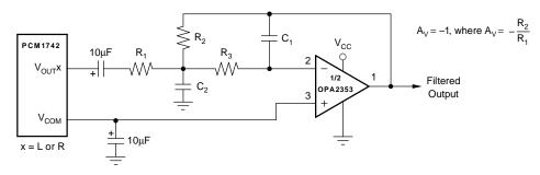
(a) Using  $V_{COM}$  to Bias a Single-Supply Filter Stage
