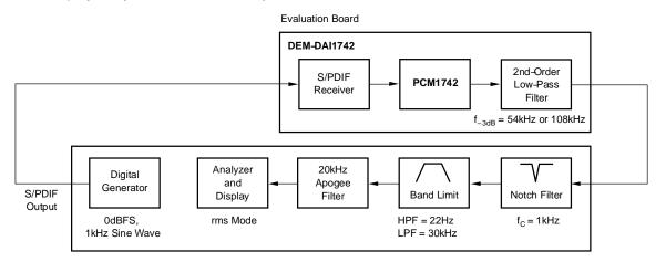
Figure 35. Test Setup for THD+N Measurements
