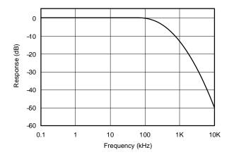
Figure 26. Output Filter Frequency Response
