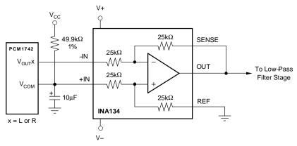
(c) Using an INA134 for DC-Coupled Output
