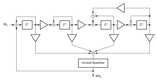
Figure 32. 8-Level Delta-Sigma Modulator
