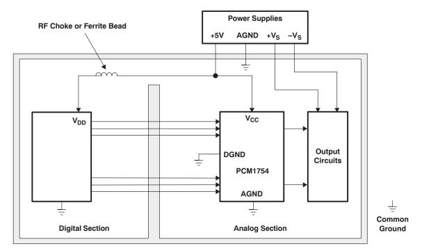
Figure 37. Single-Supply PCB Layout
