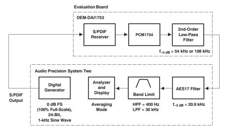
Figure 31. Test Setup for THD+N Measurement
