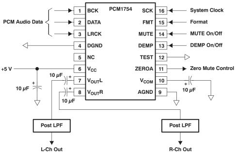
Figure 28. Basic Connection Diagram
