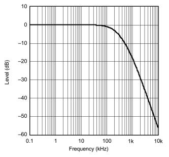
Figure 24. Output Filter Frequency Response
