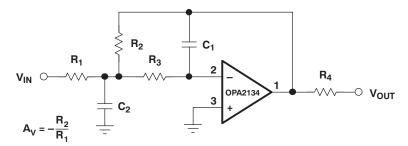
Figure 29. Dual-Supply Filter Circuit
