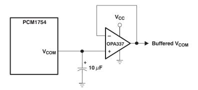
(b) Using a Voltage Follower to Buffer  $V_{\mbox{COM}}$  When Biasing Multiple Nodes
