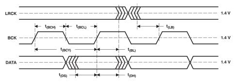
Figure 22. Audio Interface Timing
