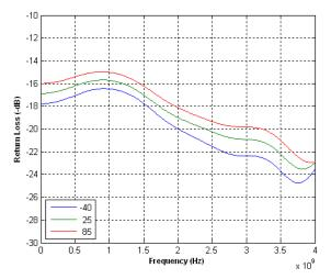
Figure 16. Return Loss: RFC @ 3.0 V
