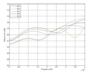
Figure 14. Return Loss at active port @ 3.0 V
