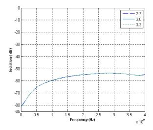
Figure 12. Isolation: RFX-RFX @ 3.0 V
