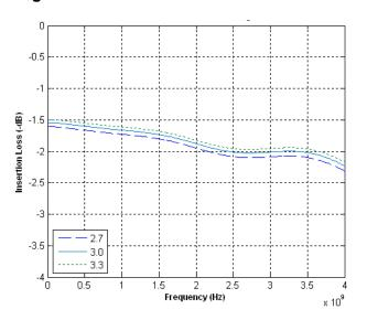
Figure 7. Insertion Loss: RFC-RFX @ 3.0 V
