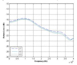
Figure 15. Return Loss: RFC @ 25 °C
