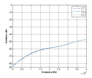
Figure 10. Isolation: RFC-RFX @ 3.0 V
