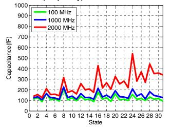
Figure 7. Measured Shunt C vs Frequency
