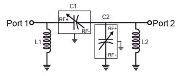
Figure 19. Recommended Layout of Multiple DTCs
