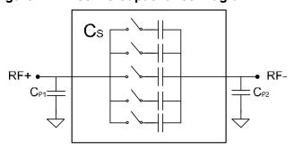
Shunt configuration (looking into RF+ when RF- is grounded) will have higher total capacitance at RF+ due to parallel combination of C<sub>s</sub> with parasitic capacitance C<sub>P1</sub> (C<sub>S</sub> + C<sub>P1</sub>), as demonstrated in Figure 15 and Table 9.
