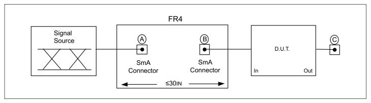
AC Test Circuit Referenced in the Electrical Characteristic Table
