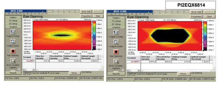
Signal Eyes at 13.8dB Input Equalization (EQ=111), 48" FR4 Input Trace and 36" Output Coax cable.
