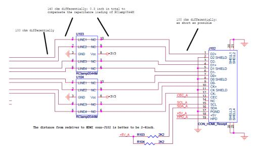
Figure 7-12 ESD Protector on PI3HDX1204B1 Source EVB
