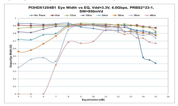
Figure 4-2 Eye Width vs. Input Equalization at Different Input trace Lengths
