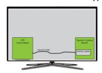
Figure 1-3 TMDS Connection Inside TV
