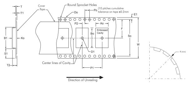
Figure 8-5 Standard Embossed Carrier Tape Dimension
