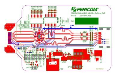
Figure 7-9 Source-side Placement near to the HDMI Connectors
