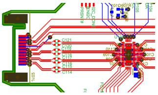
Figure 7-8 AC Coupling Capacitor Placement
