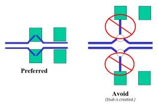
Figure 7-21 Layout Guidance of Shunt Component
