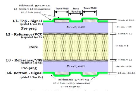
Figure 7-16 4-Layer PCB Stack-up Example
