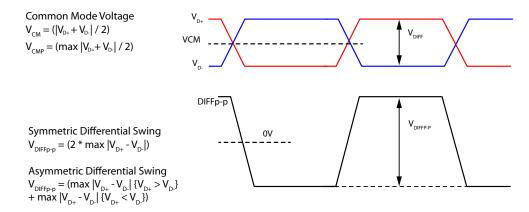
Figure 6-3 Definition of Peak-to-peak Differential Voltage
