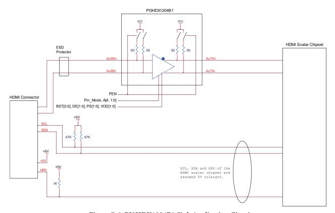
Figure 7-6 PI3HDX1204B1 Sink Application Circuit
