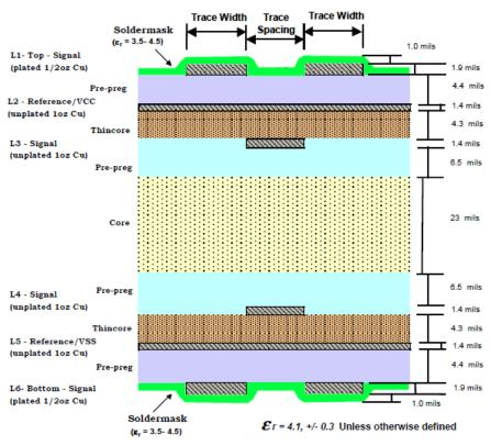
Figure 7-17 6-Layer PCB Stack-up Example
