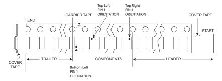
Figure 8-4 Tape leader and Trailer Pin 1 Orientation
