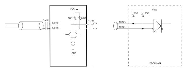
**AC-Coupled Differential Signaling Application Circuits**
