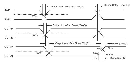
Figure 6-2 Intra and Inter-pair Differential Skew Definition
