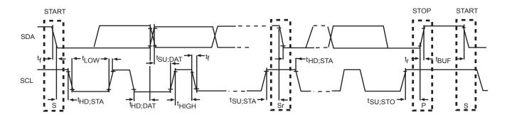
Figure 6-6 I<sup>2</sup>C Timing Diagram
