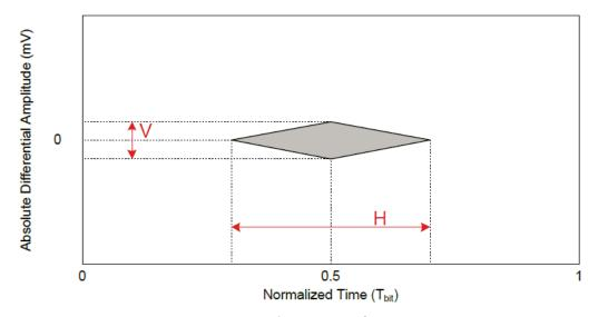
Figure 6-5 HDMI Sink Test Point for Eye Diagram
