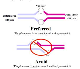
Figure 7-23 Layout Guidance of Stitching Via
