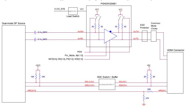
Figure 7-1 PI3HDX1204B1 Source Application Circuit
