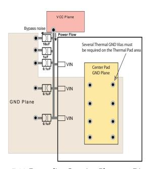
Figure 7-14 Decoupling Capacitor Placement Diagram
