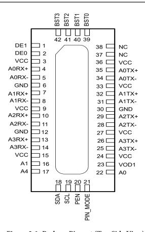
Figure 3-1 Package Pin-out (Top-Side View)
