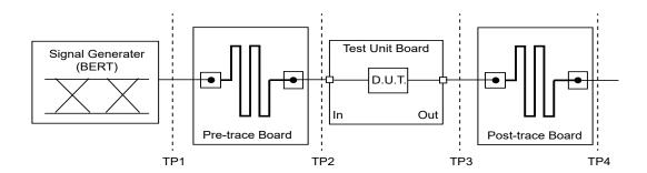
Figure 6-1 Electrical Parameter Test Setup
