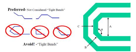
Figure 7-20 Layout Guidance of Bends
