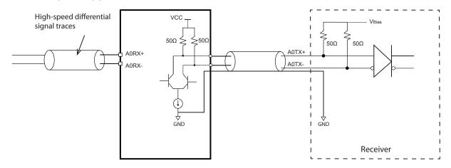
**DC-Coupled Differential Signaling Application Circuits**
