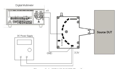
Figure 7-3 HDMI VOFF Test Setup
