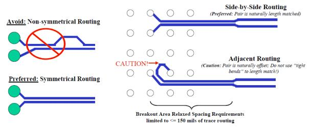
Figure 7-19 Layout Guidance of Matched Differential Pair
