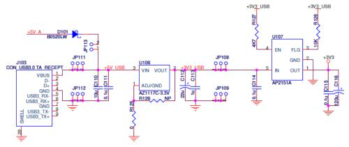
Figure 7-5 Power Distribution Switch Example
