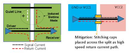
Figure 7-18 Stitching Capacitor Placement
