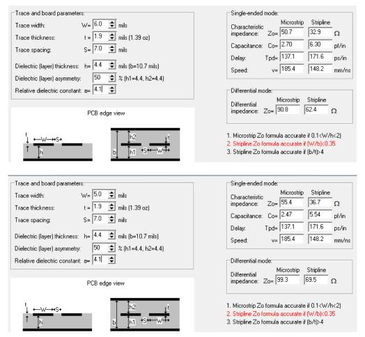
Figure 7-15 Trace Width and Clearance of Micro-strip and Strip-line
