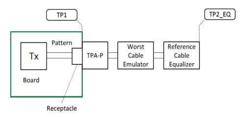
Figure 6-4 HDMI Source Test Point for Eye Diagram
