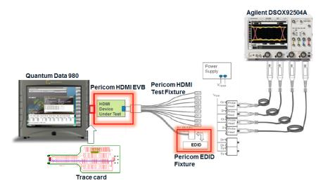
Figure 7-24 HDMI 2.0 CTS Test Setup
