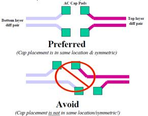
Figure 7-22 Layout Guidance of Series Component
