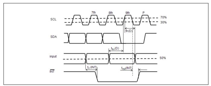
Figure 3: Timing Parameters for INT Signal
