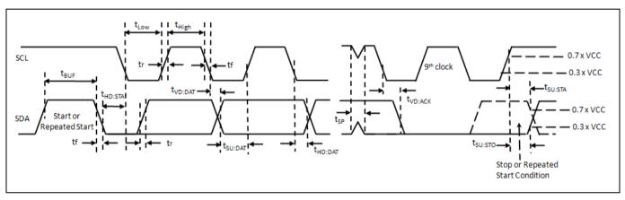
Figure 2. Definition of Timing on the I2C-bus
