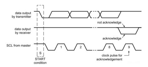
Figure 10. Acknowledgment on I2C Bus
