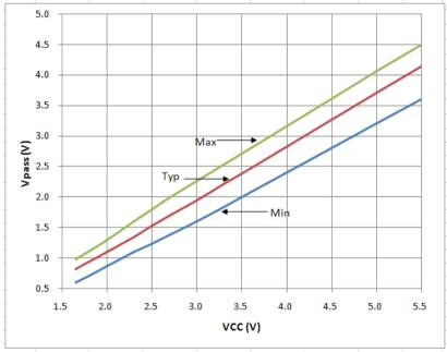
Figure 6. Vpass voltage VS Vcc
