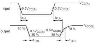
Figure 2: Propagation Delay and Transition Times B→A
