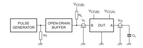
R<sub>L</sub> = load resistor; 1.35 kΩ on port B
