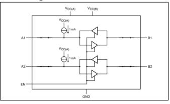
The PI6ULS5V9509 is a level translating I<sup>2</sup>C-bus/SMBus repeater. It can provide bidirectional level translation between low voltage (down to 1.1V) and higher voltage (2.5V to 5.5V) in mixed-mode applications. And it enables I<sup>2</sup>C and similar bus system to be extended, without degradation of performance even during level shifting.
