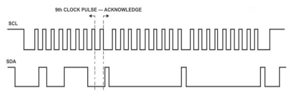
Figure 7: Bus B I<sup>2</sup>C/SMBusWaveform
