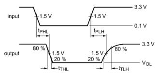
Figure 2: Propagation Delay and Transition Times
