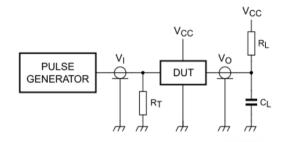
$R_L$  = load resistor; 1.35 k $\Omega$
