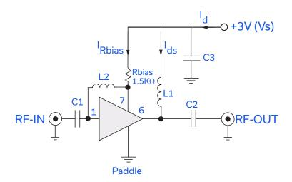
Fig 3. Recommended Application Circuit Note: Resistance of L1, 0.1- $0.2\Omega$  typically
