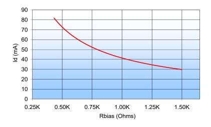
Fig 4. Id varies as a function of Rbias. The Id current range is defined based upon the specific Rbias value noted in the Application Circuit (Fig 3). Rbias may be adjusted to optimize Id for a customers' application. RF performance will vary accordingly.
