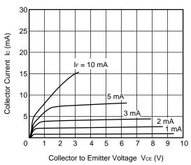
COLLECTOR CURRENT vs. **COLLECTOR SATURATION VOLTAGE**
