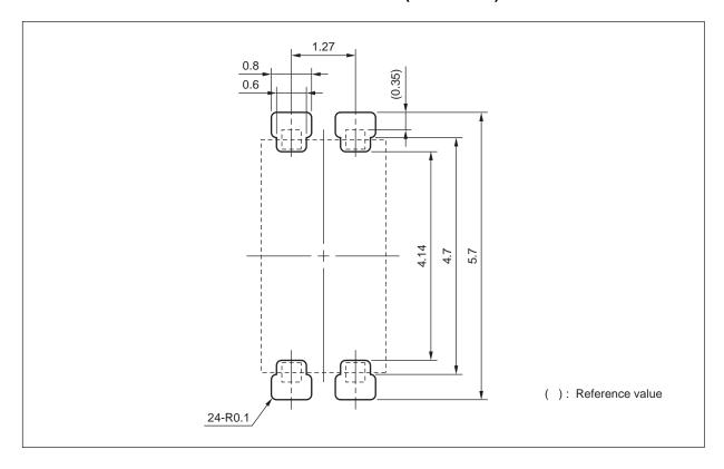
**Remark** This drawing is considered to meet air and outer creepage distance 4.0 mm minimum. All dimensions in this figure must be evaluated before use.
