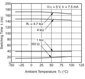
SWITCHING TIME vs. AMBIENT TEMPERATURE
