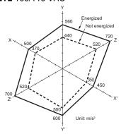
Measurement: Shock was applied 2 times each in 6 directions along 3 axes with the Relay energized and not energized to check the shock values that cause the Relay to malfunction. Criteria: Non-energized: 200 m/s $^2$  , Energized: 200 m/s $^2$
