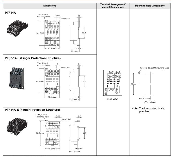
Note: If you use the PTF-08-PU, PTF-08-PU-L, PTF08A, PTF08A-E, or PT08 with an LY1 Relay, connect the following terminal pairs: 1-2, 3-4, and 5-6 (for usage at 10 A or higher).
