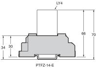
Note: 1. The PTF□A can be mounted on a track or with screws.
