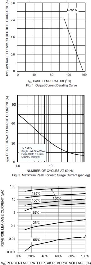
Fig.5 Typical Reverse Characteristics
