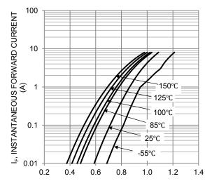
V<sub>F</sub>, INSTANTANEOUS FORWARD VOLTAGE (V) Fig. 2 Typical Forward Characteristics (Per Leg)
