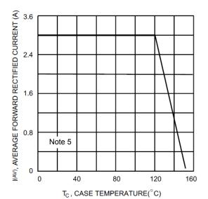
Fig. 1 Output Current Derating Curve
