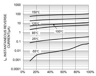
$V_R$ , PERCENTAGE RATED PEAK REVERSE VOLTAGE (%) Fig.5 Typical Reverse Characteristics
