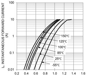
V<sub>F</sub>, INSTANTANEOUS FORWARD VOLTAGE (V) Fig. 2 Typical Forward Characteristics (Per Leg)
